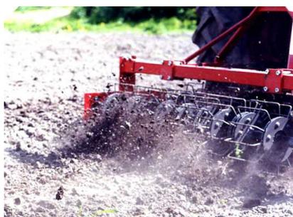
Two weeding cages in a row rotate in an adjustable depth of 1 - 4 cm in driving direction between the plant rows. The cage in front drives the rear one and also loosens the soil downwards. The second cage crumbles the soil and removes soil from the weed.
