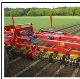
For larger working width, the maintenance-free chain-drive is mounted on both side.
