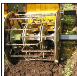
Adjustable working-elements allow with easy handling, a quick and optimal adjustment to different working and row widths.
