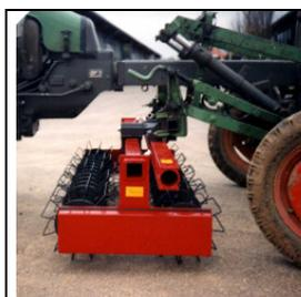
The Kress Cage-Weeder can be attached at every common Tool-Carrier
