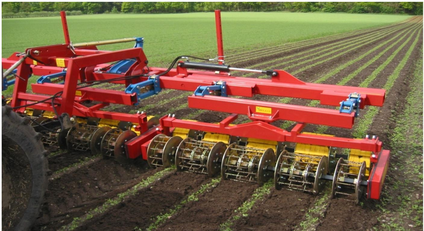
With this machine KRESS & CO had given a total new idea to mechanical weed control. The absolutely new principle of effect and construction received the award for new inventions on the Agritechnica-Show. This new method of weed control and soil loosening works particularly very effective in early stadiums. The machine is good for all row crops particularly for vegetable, special crops, medicinal and spice plants, but also for field crops like sugar beets, sunflowers etc.
