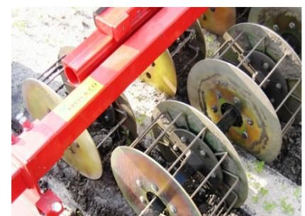
The total new tool construction causes no side pressure, therefore there is no need for row protection. Even seeded cultures can be hoed in very early stadium.
