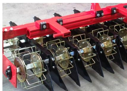
The ground driven machine is suitable for every standard tractor to mount in front, rear or between the axles. The modular concept allows quick mounting and adjusting to different working and row widths.
