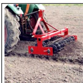
The Kress Cage-Weeder can be also used for the whole space, to prepare seed- or plant-beds
