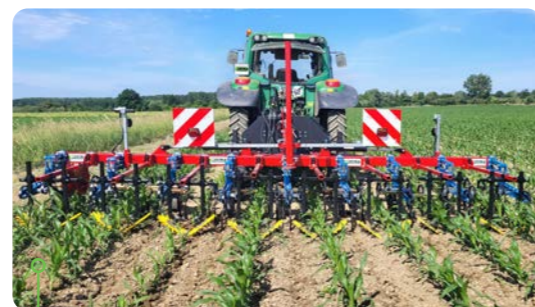
8-row weeding system for maize, with side shifting frame and 37 cm fingerweeder, yellow.
