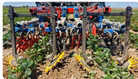
2-row strawberry weeder, combination of star cultivator and fingerweeder 37 cm, yellow.
