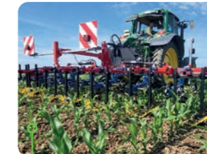
12-row hoeing system for maize, with side shift frame and 37 cm fingerweeder, yellow.
