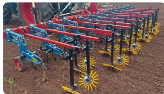
12-row weeding system for maize, with side shifting frame and 37 cm fingerweeder, yellow.
