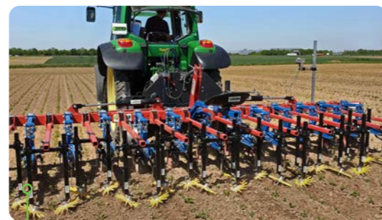
12-row weeding system for sugar beet, with side shifting frame and 31 cm fingerweeder, yellow.
